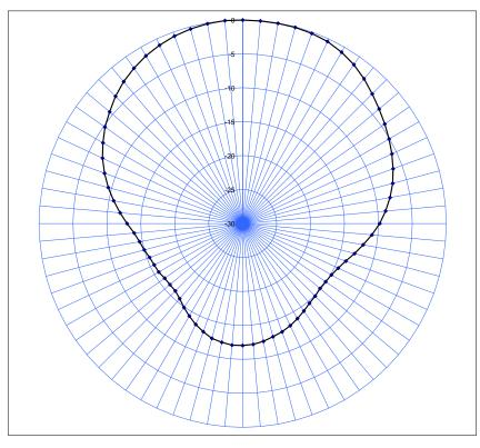
Figure 5: Typical antenna pattern of the Antenna ID ISC.ANT.U170/170-EU vertical
