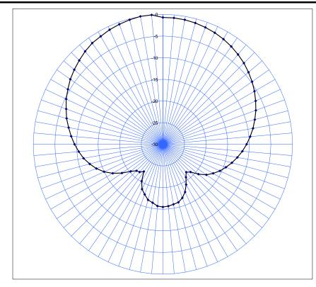
Figure 4: Typical antenna pattern of the Antenna ID ISC.ANT.U170/170-EU horizontal
