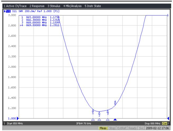
Figure 3: Typical VSWR of the antenna ID ISC.ANT.U170/170-EU
