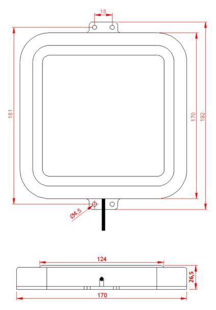
Figure 1: Mounting drawing
