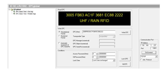
For working with one EPC transponder, the item **EPC Class 1 Test – One Tag** must be selected. The dialog window allows the **Write**, **Lock** and **Kill** of an UHF-EPC transponder. For HF-EPC transponders, only the **Write** button is accessible.
