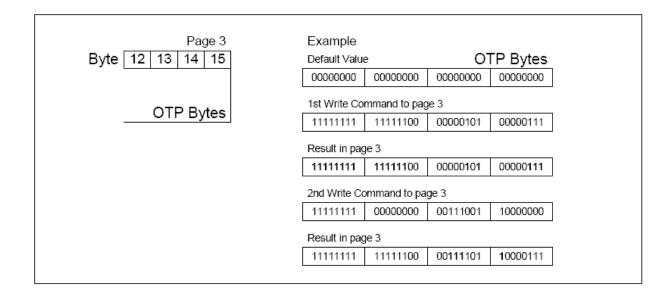
The bytes of the write command and the current contents of the OTP bytes are bit-wise "or-ed" and the result becomes the new contents of the OTP bytes. This process is irreversible. If a bit is set to "1", it cannot be changed back to "0" again.
